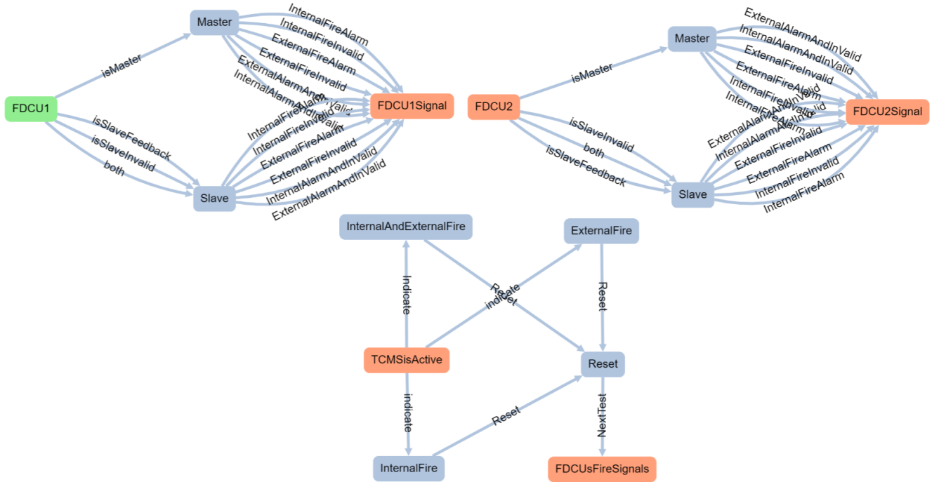
Figure 6. Final FSM-based shared model with multiple diagrams created from requirements and test specifications having shared nodes
