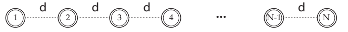
Fig. 3. Illustration of a regular line network in which the distance between two adjacent nodes is d .
