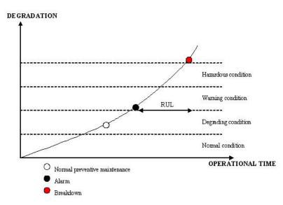
Figure 2: The normal preventive maintenance is often carried out before the component, sub-system or system is showing any signs of fault. With the CBM technique one often say "If it ain't broke, don't fix it". RUL is an abbreviation of Remaining Useful Life.
