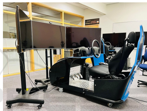
Figure 2: The car simulator developed with DriverSeat 650 ST was used for conducting the simulation tests.
