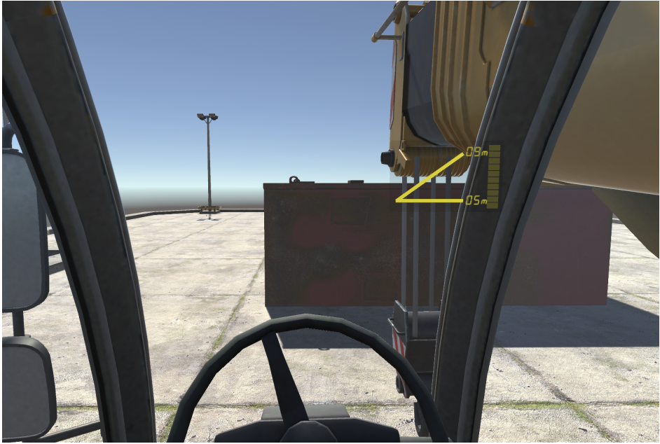
Figure 5.5: The view taken from inside the cabin of the virtual mobile crane. We placed the visualization that indicates the relative lifting capacity on the right side of the front windshield.
