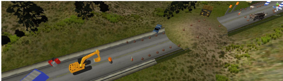
Figure 4.3: The bird's-eye view of the virtual environment used in the A/B test. The participants had to drive the virtual excavator, while trying to avoid colliding with any obstacles. This figure also appears in Paper B [162].
