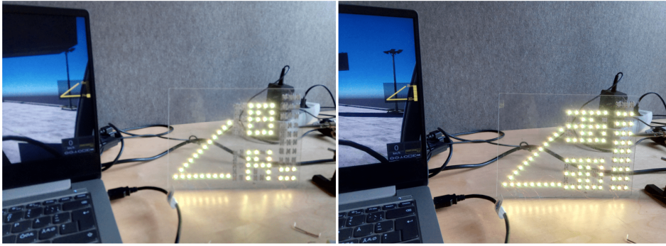
Figure 5.7: The examples that show the integration between the virtual transparent display and its physical counterpart. The physical prototype would present the same information as the information presented on the windshield of the virtual mobile crane. This figure also appears in Paper F [135].
