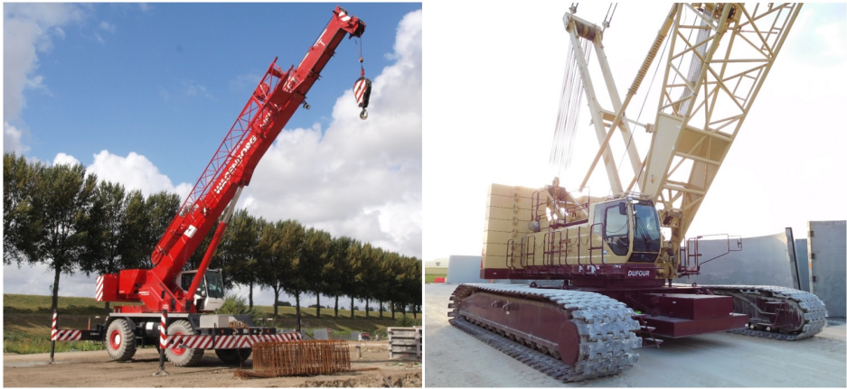
Figure 1.2: The left image shows a wheeled crane [157, CC0 1.0], while the right image shows a crawler crane [17, CC BY-SA 4.0].
