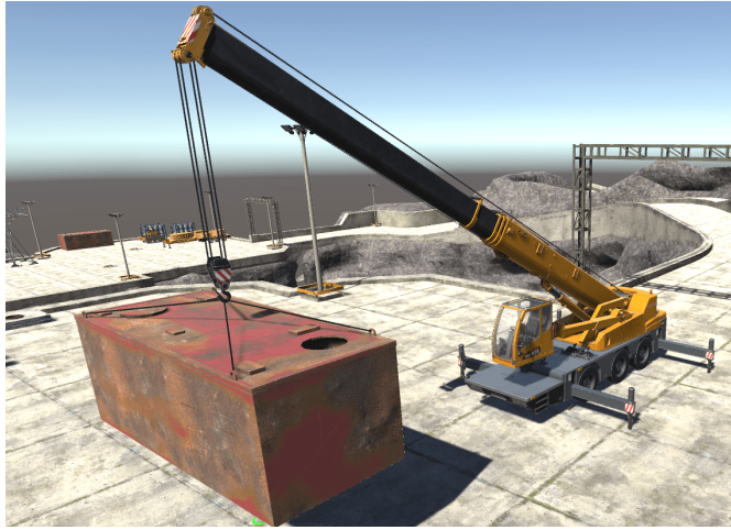
Figure 4.11: The virtual mobile crane that exists inside the simulation. The virtual mobile crane closely resembles the Liebherr LTC 1050-3.1 crane [86]. This figure also appears in Paper F [135].
