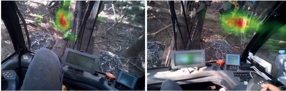
Figure 1.1: The left image shows the heat map of eye fixations when felling a tree, while the right image shows the heat map of eye fixations when cutting a tree into smaller logs [149, CC BY-SA 4.0]. The colors change from green to red based on the fixation frequency (from low to high) on specific areas. The images were taken from a forest harvester’s cabin.
