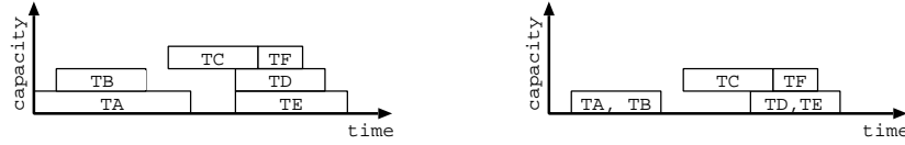
Figure 4.2: The number of binary overlaps of the infeasible schedule for a cumulative-1 constraint with capacity 2 is equal to the cost of the serialized constraint on the right, where some tasks have been merged.
