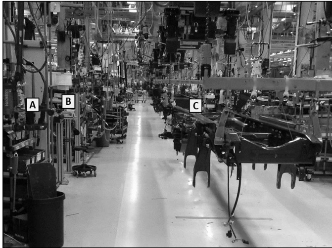
Figure 10 Existing gearbox suspension assembly station. The suspension is moved from incoming material rack (A) to preassembly station (B) to be assembled on the frame (C) (Paper E).
