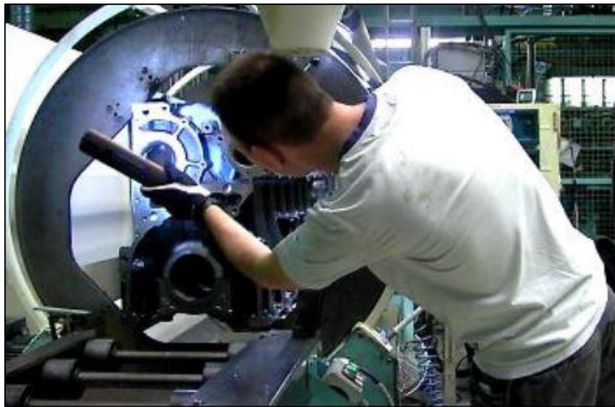
Figure 8 Current visual inspection system. The operator inspects the side of the engine block; the circular frame surrounding the block is used to rotate it to enable inspection of the side surfaces (Caliskan and Khalid, 2015).
