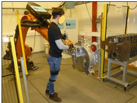
Figure 17 Physical experiments in which the motion capture system collects joint data (Paper B).
