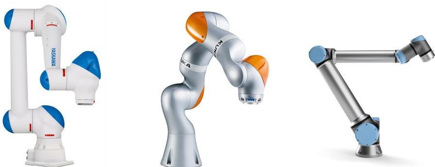
Figure 3 Examples of power- and force-limiting robots Motoman HC10, KUKA lbr iiwa and UR10e.
