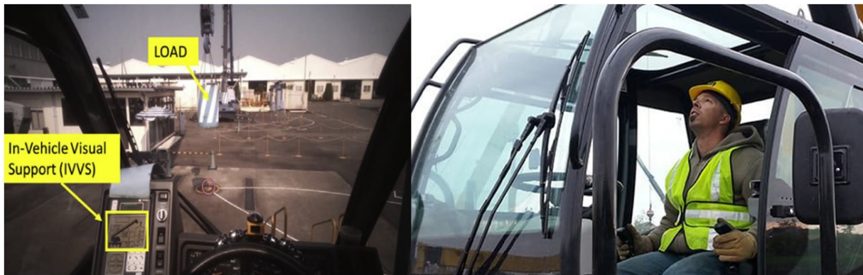
Figure 1: The left image shows an example of supportive system inside a mobile crane [6]. The right image illustrates that mobile crane operators often look at areas that are far away from the location where the supportive system is placed [2].
