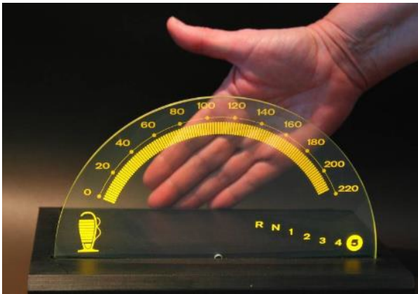
Figure 4: An example of stand-alone transparent display [1]. Each fixed element can be individually lit, whereas the widget's structure is statically rendered in the material.
