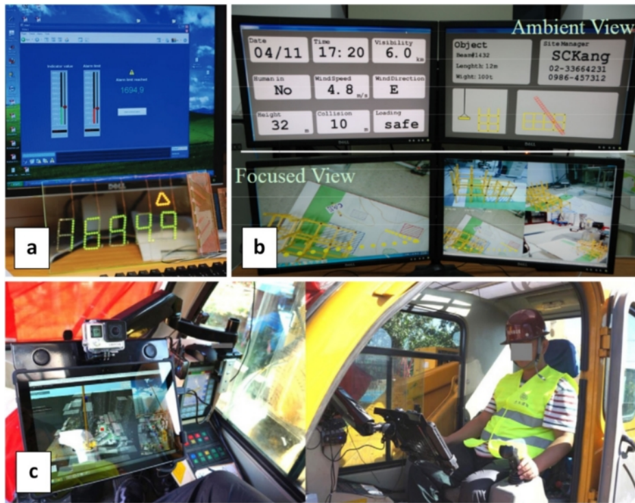
Figure 2: a. The transparent display that could be installed on the crane's windshield [14]. b. Using multiple displays for operating remote tower cranes [4]. c. Operating a mobile crane through a tablet-like display [11].
