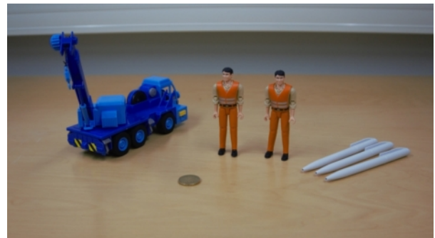
Figure 5: The tools that were used to test the operators' understanding on the proposed visualization concepts. The human toys were used to represent nearby obstacles, the coin was used to indicate where the machine's center of gravity is, and the pens were used to indicate both wind speed and direction.
