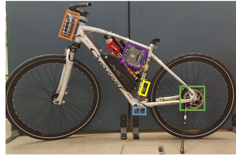
Fig. 6. The instrumented bicycle with its rear wheel motor inside the green square. The blue box indicates the position of the VN-100, used for measuring the lean angle. Inside the yellow box is the electrical speed controller. National Instruments roboRIO is mounted on the bicycle and is highlighted by the purple box. To be able to send remote commands to the bicycle, the receiver inside the red box is utilised. The motor used to control the steering angle is highlighted by the orange rectangle.
