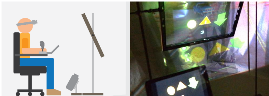
Fig. 5. To the left, a schematic picture of the CAVE simulation room and its primary components. To the right, a photo that shows all three display solutions at once (the simulation only showed one at a time)
