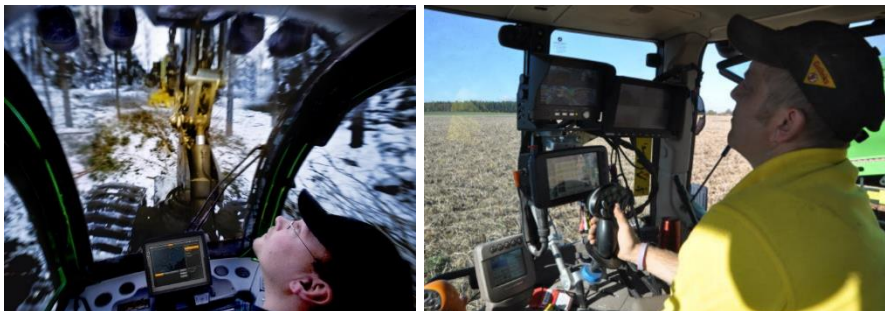
Fig. 1. To the left, a cabin with large windscreens for good visibility. To the right, an example of a cabin with four displays covering the windscreen, including one display which is not visible
