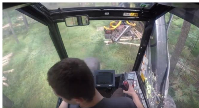
Fig. 5. The operator was turning his body when reversing the forest harvester [31].
