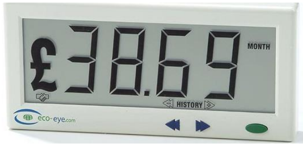
Figure 1 – The Eco-Eye: displaying the price of current energy consumption in a household 1
