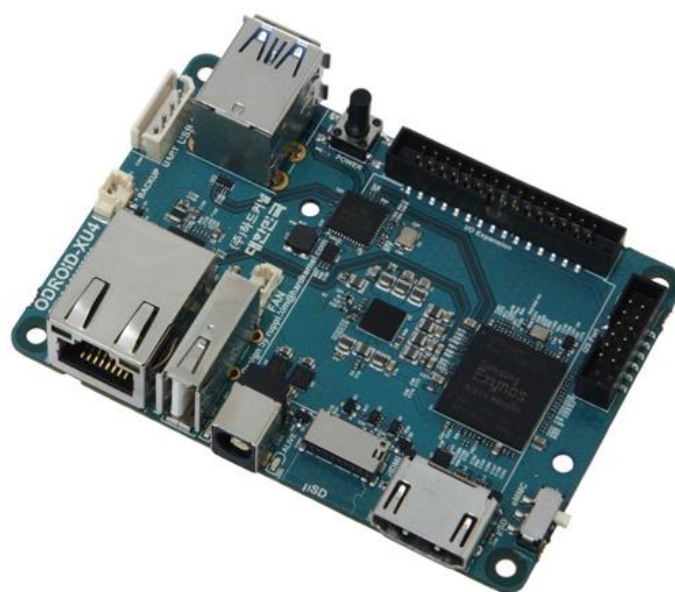
Figure 7. ODROID appearance and interfaces, as depicted in [36].
