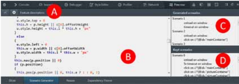
Figure 8.3: Scenario Generator used as a Firefox plugin. A – toolbar; B – web application code; C – Generated Scenarios; D – Kept scenario
