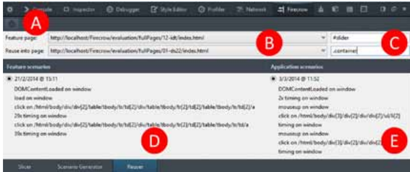
Figure 8.4: Feature Integrator used as a Firefox plugin. A – toolbar; B – Setting the feature and the target page; C – Specifying the parts of the page structure that define the feature and the position where the feature will be reused; D – Feature scenarios; E – application scenarios
