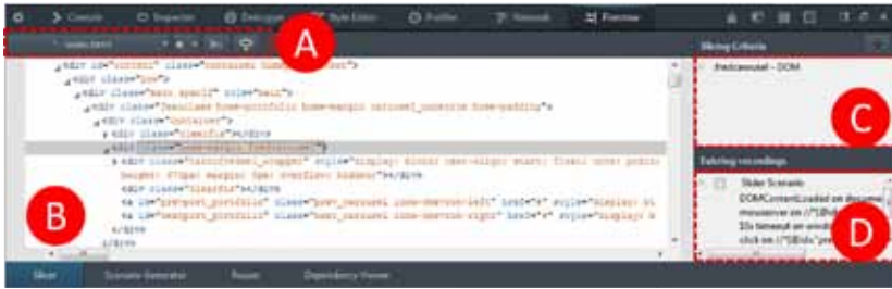
Figure 8.2: Feature Locator used as a Firefox plugin. A – action toolbar; B – DOM viewer; C – Slicing Criteria; D – Scenario description
