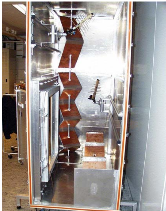
Figure 1. The basic Reverberation Chamber with dual mode stirrers.
